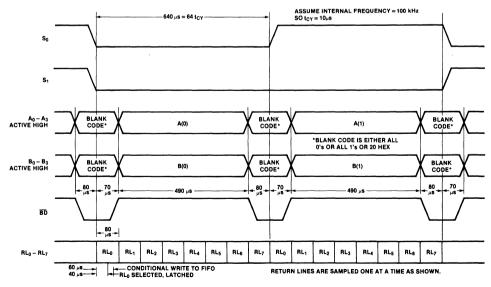
NOTE: SHOWN IS ENCODED SCAN LEFT ENTRY  $S_2 \cdot S_3 \text{ ARE NOT SHOWN BUT THEY ARE SIMPLY } S_1 \text{ DIVIDED BY 2 AND 4}$
